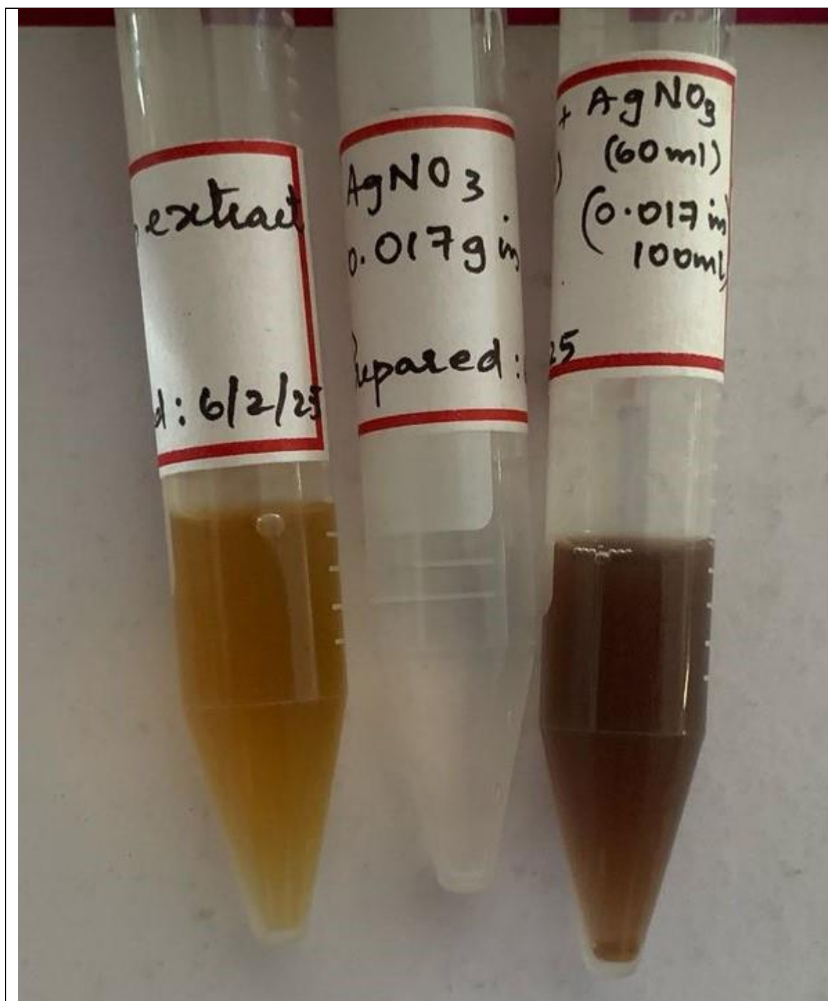
Figure 2. Visual observation of silver nanoparticle (Ag-NP) formation: Azadirachta indica extract; (Left) silver nitrate solution (middle) and (C) silver nanoparticles. (Right)
